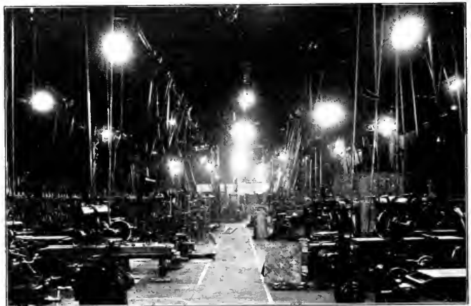
FIG. 4 EXPENSIVE MACHINERY BUT SCANT LIGHT AND VENTILATION Rapid and Accurate Work Is Possible in Such Surroundings
